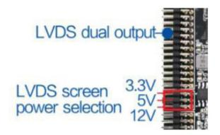
The jumper cap is used to select the screen power, from top to bottom, followed by 3.3V/5V/12V
