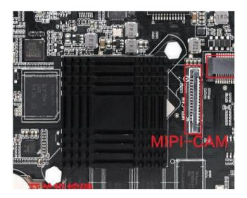
The card maximum supports a 1400w pixel mipi camera, installed in the jp26 socket, the electrical definition of which is as follows
