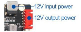
The power socket interface is defined as follows: power board is used to supply power, and the sub standard is 4Pin 2.54mm spacing
